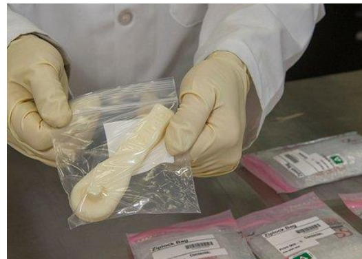
Wrench printed in space is tested at NASA Marshall SFC. Credit: NASA / MSFC / Emmett Given
